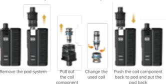
Coil Installation (Pod For BP Coil):
